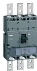
Reg. Electronico H3+ h1000 3P (320-800A) LSI, 85kA/240V
